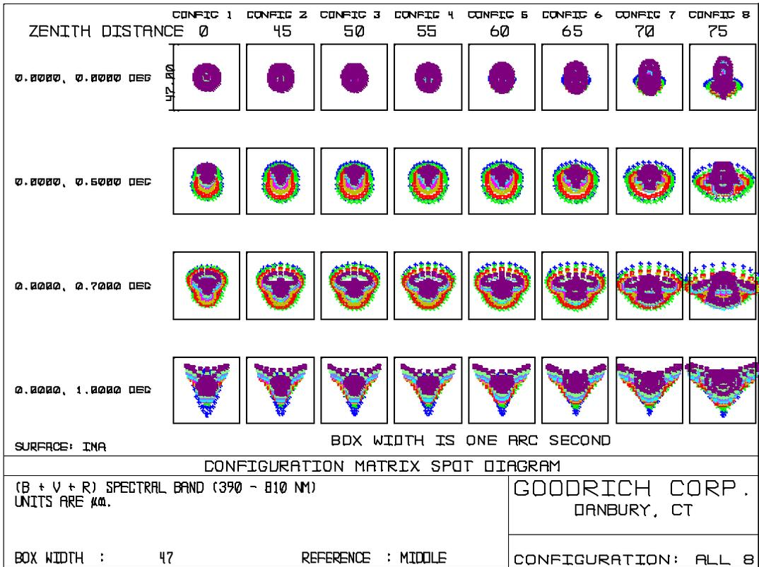
Figure 3. Spot Diagrams Showing Performance of the ADC.
