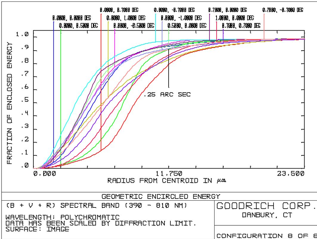
Figure 5. Encircled Energy Curves at 75° Zenith Distance.
