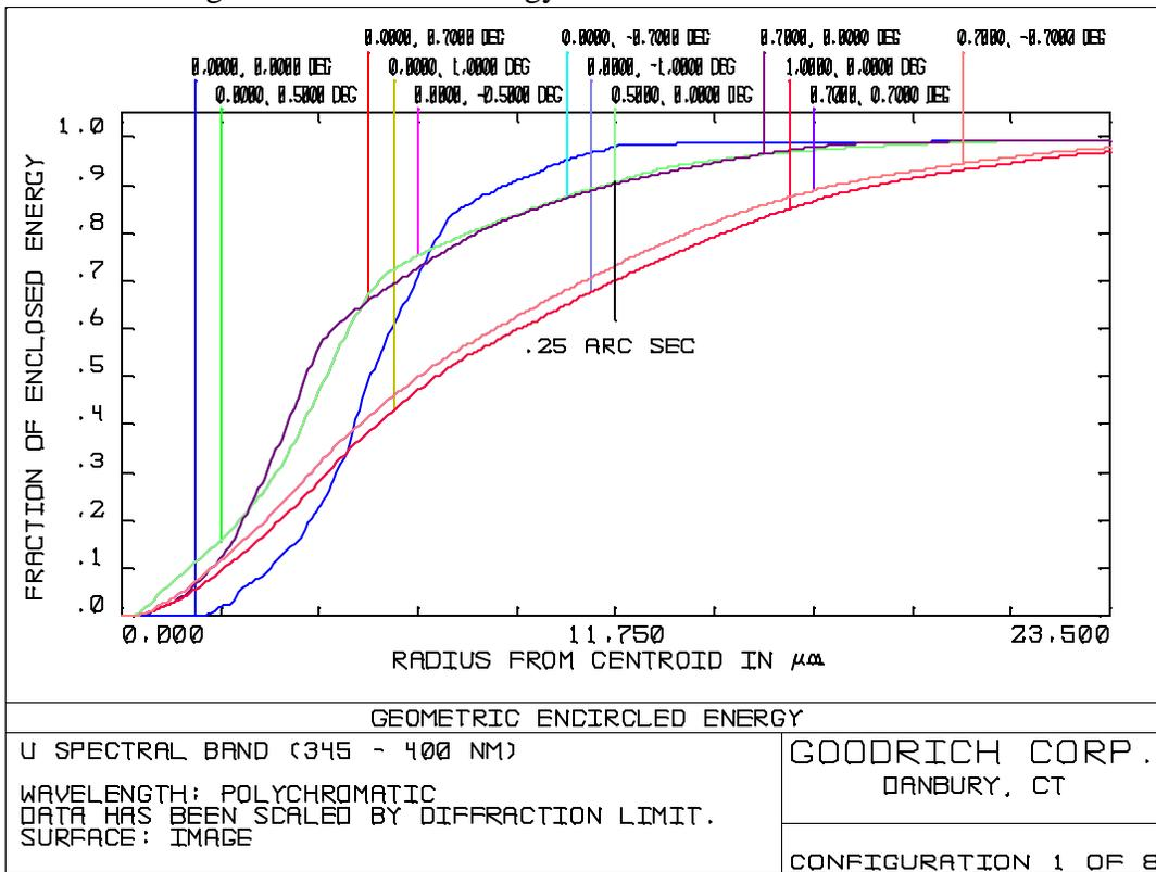
Figure 6. U-Band Encircled Energy Curves at Zenith.
