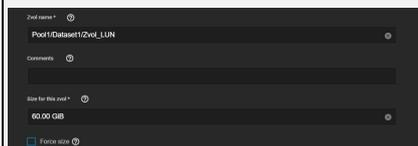
TrueNAS prevents data loss by not allowing users to reduce the Zvol size. TrueNAS also does not allow users to increase the Zvol size past 80% of the pool size.
