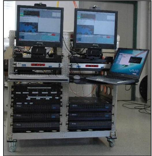
Fig. 1. The instrument, complete except for final cable routing, is shown mounted on the SOFIA telescope during ground operations in 2004 (left) and the completed instrument control rack is shown in the lab (right). The laptop computer on the keyboard tray is not part of the rack configuration, but demonstrates that the tray can carry this load.
