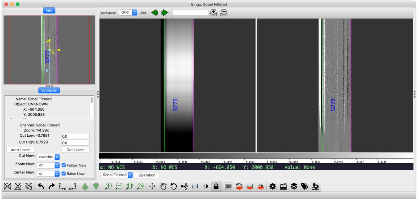
Figure 34: Example of output from the `pypeit_chk_edges` script for data taken with the DV2 grating. The magenta and green lines in the center panels mark the left and right edges of the detected slit. The CCD is about 2'9 wide, so at least one edge of the 2'5 slit should be visible.
