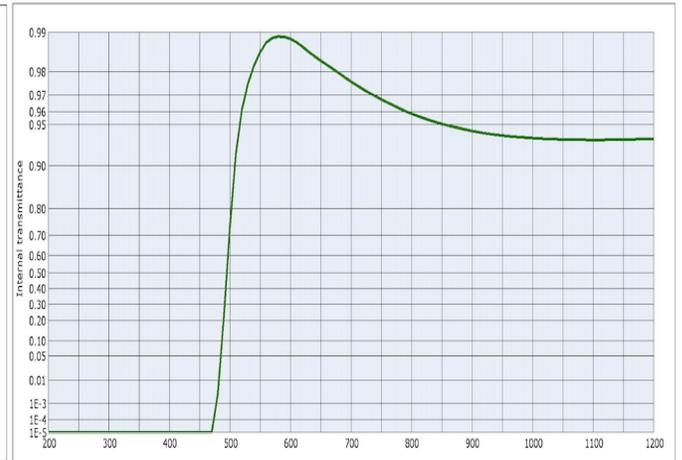
(b) GG495 filter transmission curve (from Schott).
