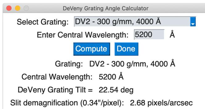
Figure 6: Grating angle calculator GUI. Select the installed grating from the drop-down, enter the desired central wavelength, and press `Compute`.
