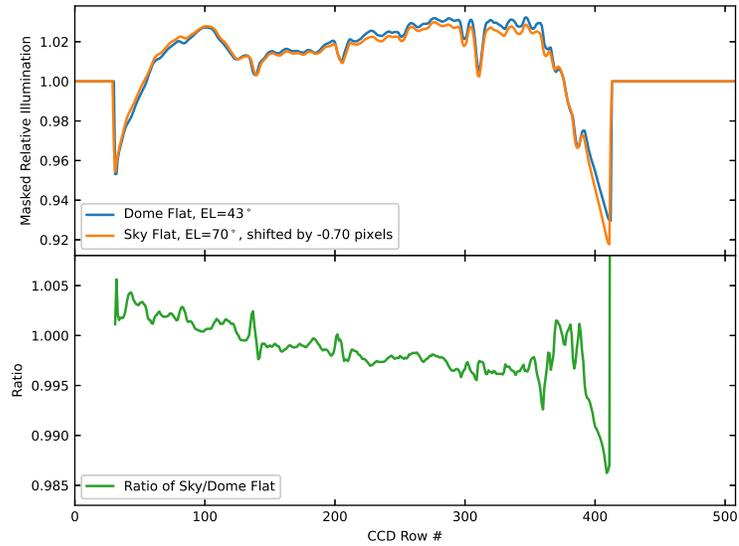
Figure 30: Slit illuminations functions for dome and sky flats for the DV3 grating. Data taken 2021-10-31UT. In the top panel, the sky flat (orange) was shifted by  $-0.7$  pixels to align the features in the illumination functions. The bottom panel shows the ratio of sky:dome flat illumination functions to gauge the differences between sky illumination (identical to science frames) and that cast by the cloverleaf pattern of the top-ring lamps. Answer: they generally match to within 0.5%.
