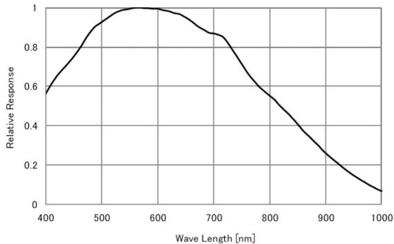
Figure 21: Typical CCD response curve for a Lodestar X2.
