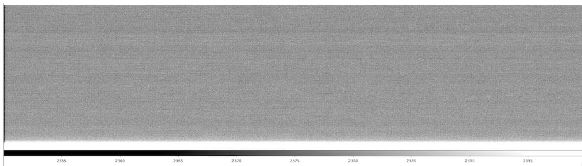
Figure 9: Example of a well-behaved bias frame (2020-12-14UT). Some bias frames will display a remaining low-level ( $\pm 2$  DN), time-variable noise pattern, which may affect low-SNR spectral extractions.
