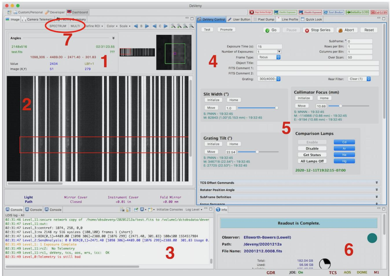
Figure 2: The layout of the DeVeney LOUI. 1: This area gives information about the currently displayed (*i.e.*, previously exposed) image. 2: Displays the spectral images, blue on the right, red on the left. 3: lois log. 4: CCD/Instrument control panel. 5: Control for spectrograph hardware and comparison lamp power. 6: Info tab, contains directory information and information about the current exposure. 7: Analysis tools.
