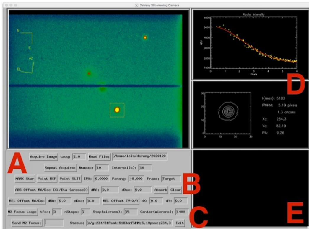
Figure 14: IDL slitviewgw control GUI
