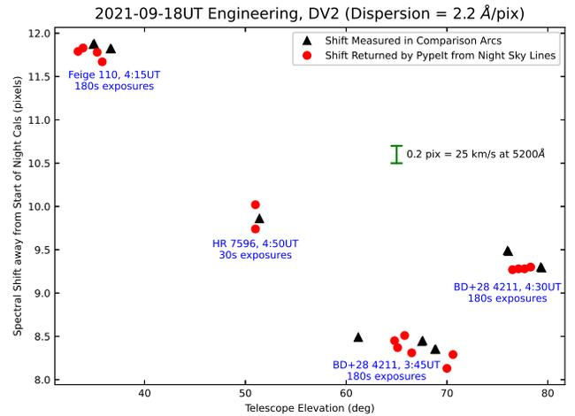
(b) Comparison of directly measured and PypeIt-derived spectral line shifts away from zenith-pointing comparison arcs
