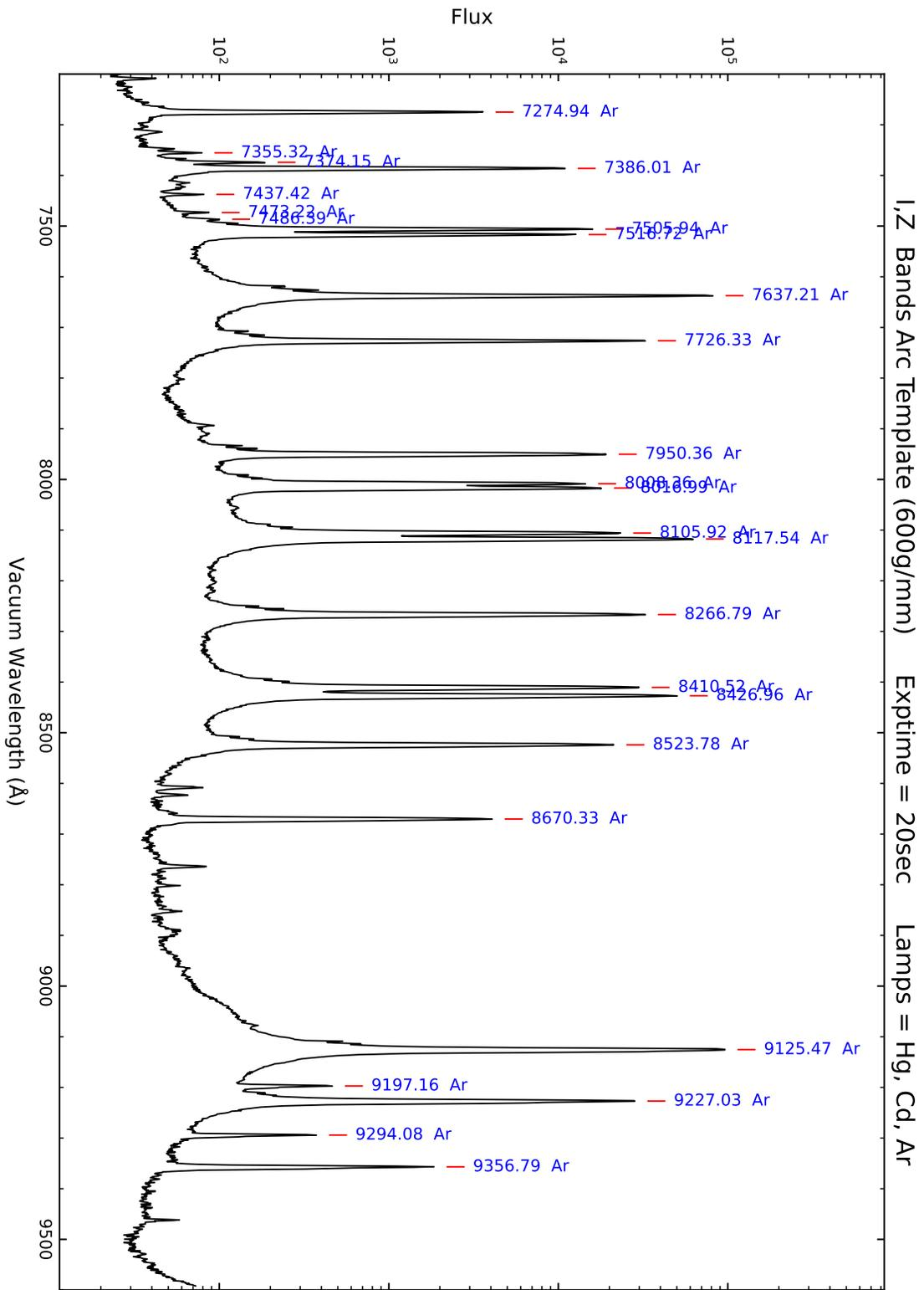
Figure 26: Line identification plot covering the wavelength range 7200 Å – 9600 Å (taken with the DV7 grating), shown on a log scale to emphasize weak lines. Enabled lamps: Argon, Mercury, and Cadmium. The OG570 blocking filter is in use to limit lines to first-order spectra only.
