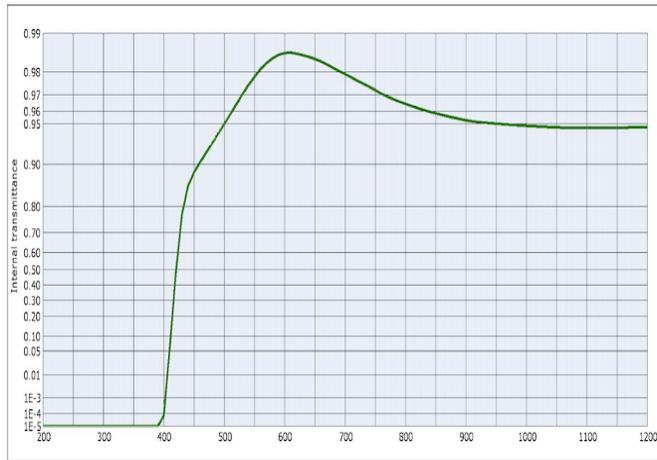
(a) GG420 filter transmission curve (from Schott).
