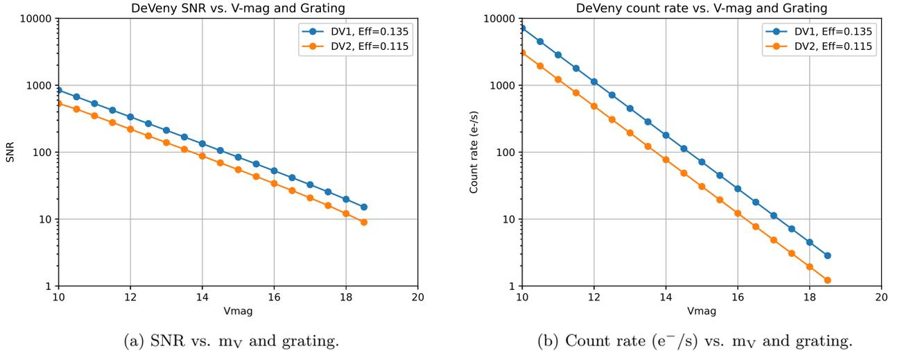
Figure 22: *Left*: SNR vs. V-mag and grating, at 5400Å system efficiency and 100 s exposure time. *Right*: Count rate (e<sup>-</sup>/s) vs. V-mag and grating, at 5400Å system efficiency.
