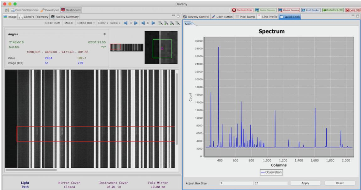
Figure 4: Use of the SPECTRUM tool. In the top portion of the DeVeney LOUI, in the left panel a region (red rectangle) has been selected via click-and-drag. In the right panel the “Quick Look” tab is selected and the mean spectrum (averaged over rows) for the selected region is displayed here.
