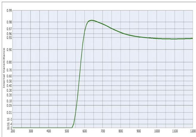
(c) OG570 filter transmission curve (from Schott).
