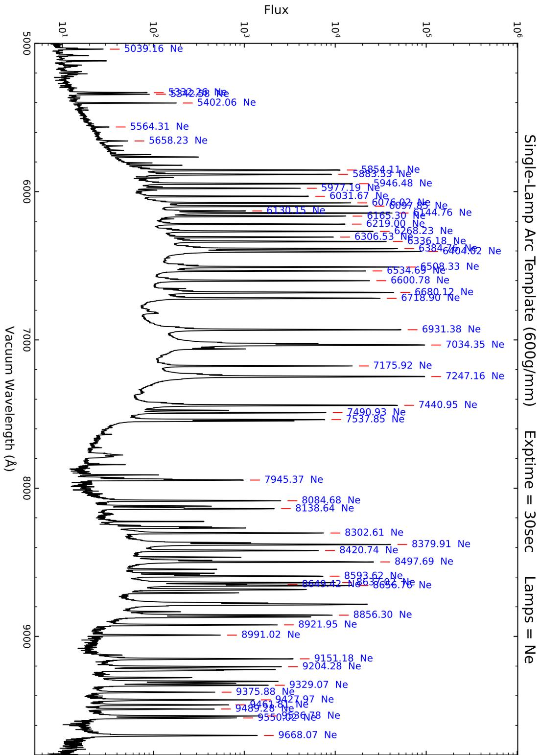
Figure 27: Neon-only line identification plot covering the wavelength range 5000 Å – 9800 Å (taken with the DV6 & DV7 gratings), shown on a log scale to emphasize weak lines. The GG420 (5900Å < λ < 7850Å) and OG570 (λ > 7850Å) blocking filters are in use to limit lines to first-order spectra only.
