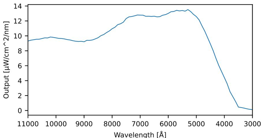
Figure 19: Manufacturer’s spectral power distribution curve for the SoLux 4700K (“Top Ring”) lamps. The abscissa is drawn with blue to the right to match how spectra appear on the CCD.
