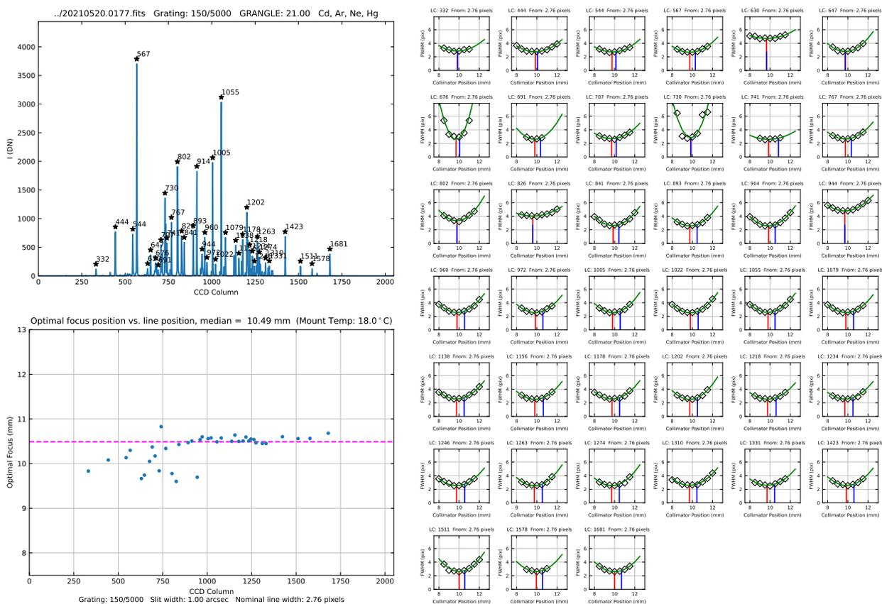
Figure 8: Example output plots from `dfocus` analysis for DV1. *Upper left:* Arc line plot. *Lower left:* Optimal focus vs. line position plot. The median value is 10.49 mm. *Right:* Individual line focus curves.
