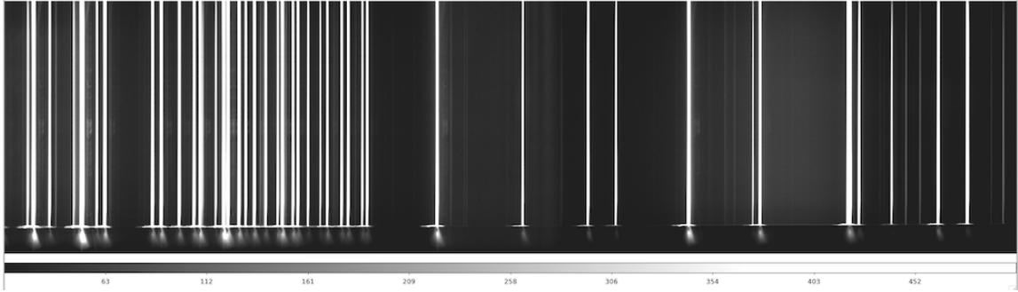
Figure 10: Example arc frame, taken with the DV2 grating at a central wavelength of 5200Å. Lines are from all four lamps (Ne, Ar, Hg, Cd). Wavelength coverage is approximately from 7350Å on the left to 3000Å on the right.
