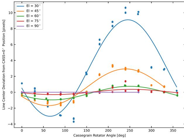
(a) Spectral shift of arc lines as a function of telescope elevation and cassegrain rotator angle
