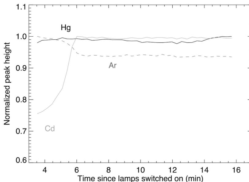
Figure 18: Arc lamp warm up curves. Ne and Ar brightnesses stabilize within a minute, Hg in 1-3 minutes, and Cd in about 6 minutes. They may well be usable before fully stabilized, but caveat emptor. (Courtesy: N. Moskovitz)
