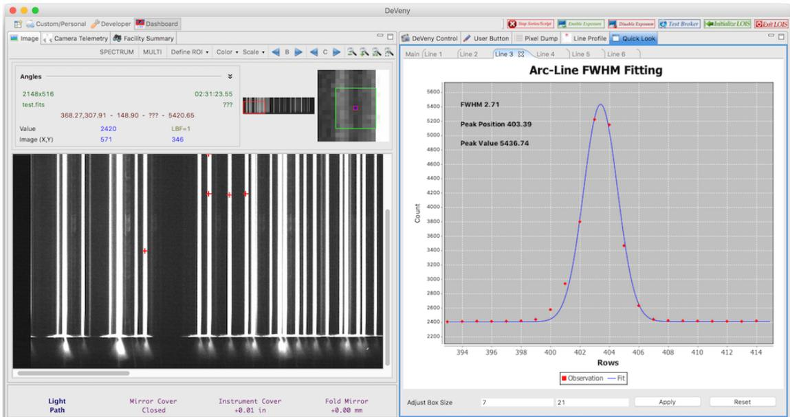
Figure 5: Use of the MULTI tool. In the top portion of the DeVeney LOUI, in the left panel several lines have been selected. In the right panel the “Quick Look” tab is selected and each line is plotted in its own tab. The tabs display the data points, a fit to the selected line and a few statistics. (NOTE: While the abscissa is labeled as “Rows”, it is actually plotting column number. This is a bug in the LOUI.)
