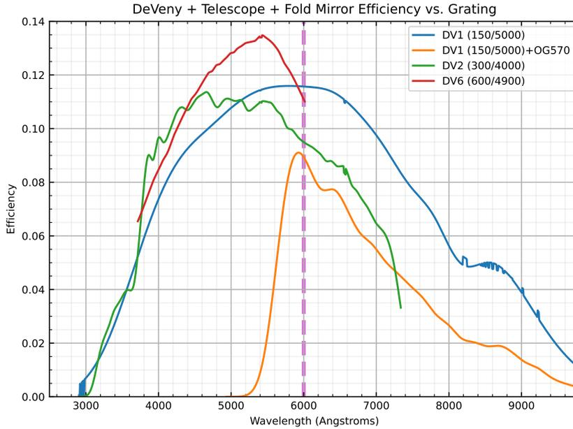
Figure 17: On-sky measured DeVeny efficiency vs. wavelength for several gratings. The vertical line at  $6000\text{\AA}$  shows where 2<sup>nd</sup>-order leakage would begin for unfiltered spectra. The spectra were all taken with a  $5''$  wide slit. Blue: DV1, no filter, 2022-04-14, BD+33 2642. Orange: DV1, OG570, 2022-04-15, BD+33 2642. Green: DV2, no filter, 2015-05-07, Feige 66. Red: DV6, no filter, 2022-02-05, G191-B2B.
